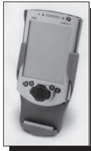
Figure 17—Most personal digital assistants have only one expansion slot. This expansion pack contains a radio, laser scanner, and separate power pack, transforming a normal PDA into a wireless bar-code scanning dynamo.
