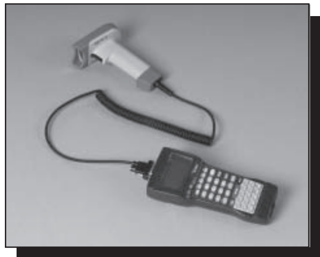
Figure 13—This portable data terminal uses an RS232 connection to a laser bar-code reader.
