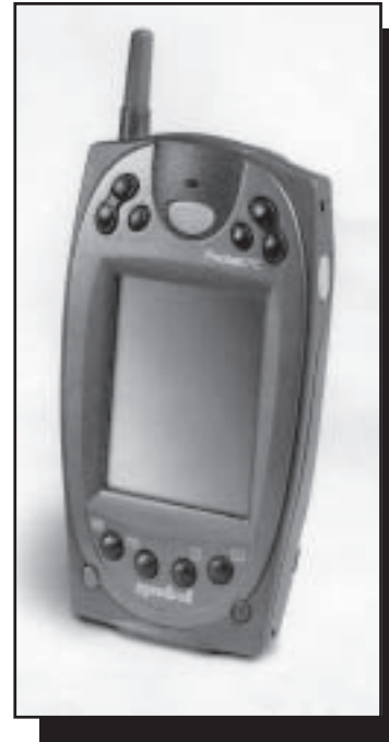
Figure 16—This wireless personal digital assistant contains an internal radio, freeing the expansion slot for a bar-code scanning card.
