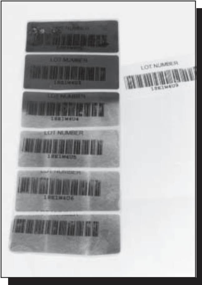
Figure 3—These labels turned black after an hour of exposure to direct sunlight. A fresh label (right) is shown for comparison.
