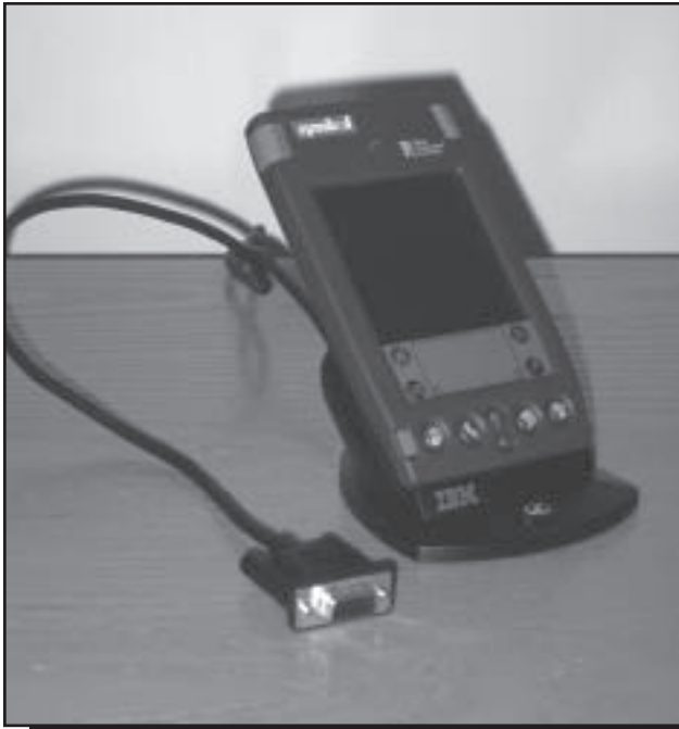
Personal digital assistant configured for bar-code scanning with the docking terminal and cable system.
