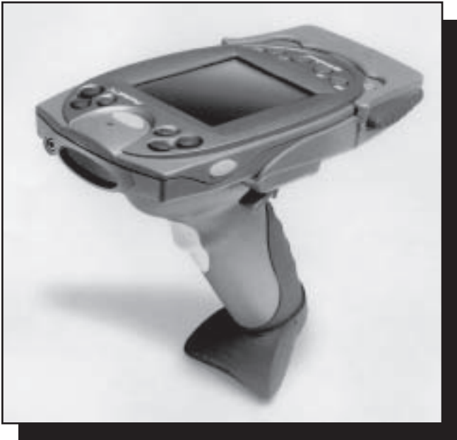
Figure 18—Using a personal digital assistant to scan bar codes can cause hand fatigue. Handle adapters are available for many models.
