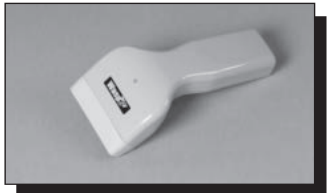
Figure 11—A CCD reader is a good choice when you don't need to scan from a distance.
