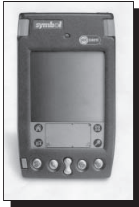
Figure 14—The Symbol SPT 15xx model series are popular entry-level personal digital assistants with an integrated laser bar-code reader.
