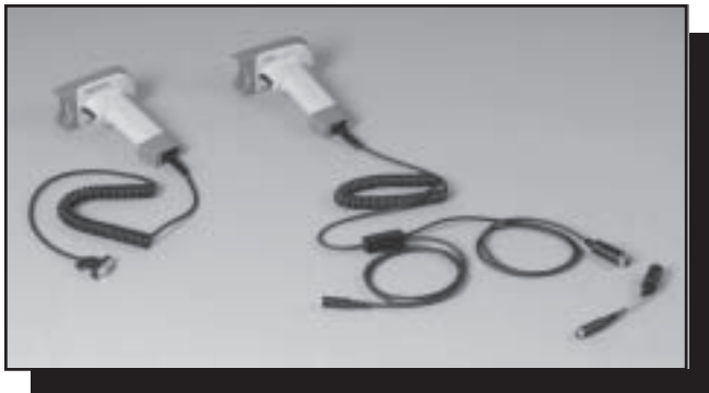
Figure 7—These two readers are the same model, but use different methods of connecting to a computer.
