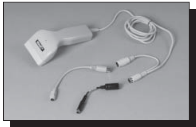
Figure 8—This CCD (charge-coupled device) bar-code reader uses a keyboard “wedge” cable configuration.
