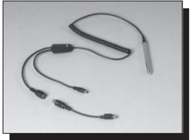
Figure 10—This wand reader uses a keyboard wedge cable. The separate cable is an adapter for older IBM-compatible models.
