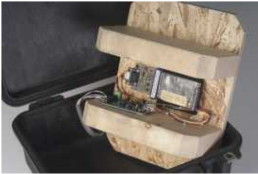
Figure 2 —The TRAFx bicycle counter was placed in a Pelican case.
