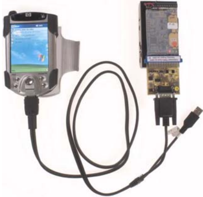
Figure 4 —A personal digital assistant (PDA) can be used to program the TRAFx Research mountain bike counter.
