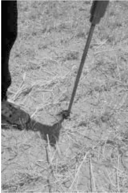
Figure 7.5. Gently rotating or tapping the penetrometer at the soil surface can help remove it.
