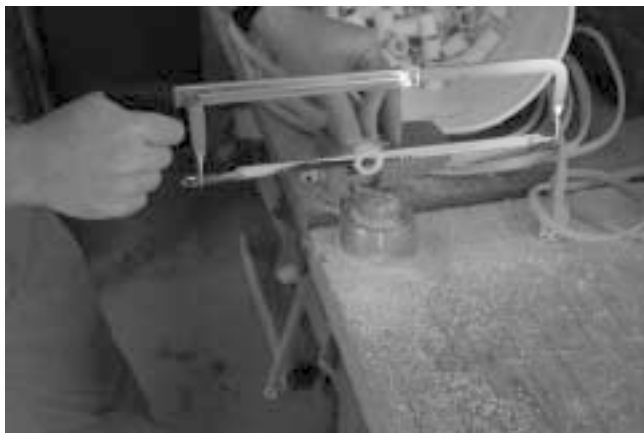
Figure A.1. First cut on PVC.
