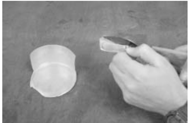
Figure A.5. Cutting shovels with tin snips.
