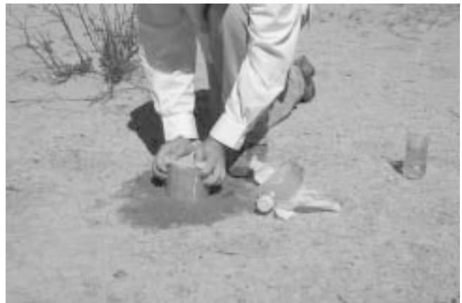
Figure 8.4. Insert infiltration ring to 3 cm.
