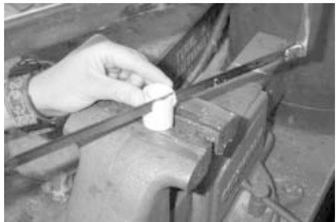
Figure A.2. Second cut on PVC.
